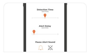
**5.** The Alert Delay period is a time where the Core will be beep rapidly and the control switch will flash red. This is an indication that a tag is about to set of the MOB alarm. During this period if the tag is brought back into range the alarm is automatically canceled. This can be a very helpful setting to help test the limits of your setup.
