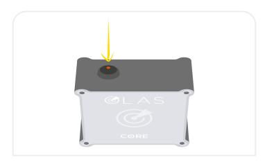
**3.** Cancel the alarm on the Core by pressing the control switch once.
